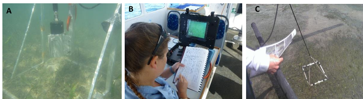
Figure 7. Methods for mapping and monitoring seagrass for subtidal meadows using (A, B) digital camera mounted on a drop frame connected to CCTV, and for intertidal meadows (C) helicopter aerial surveillance.
